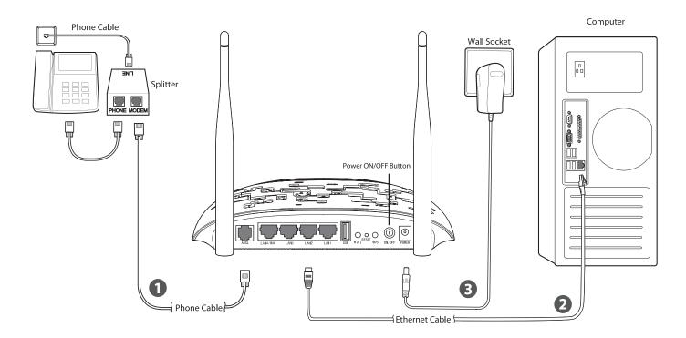
Press the **ON/OFF** button of your modem router and make sure the LEDs (especially the ADSL LED) display as shown below.
